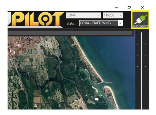
Once connected the Flight Controller parameters will be read, and available to view/modify (the first time connecting will take longer as all the parameters are downloaded).
