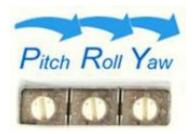
The gain values can be adjusted directly on the Gyro with the small screwdriver provided, when on the ground; clockwise to increase and anti-clockwise to decrease as indicated.
