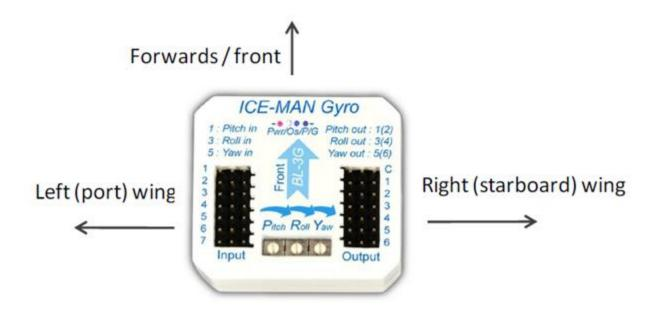
The modified Bluelight Technologies ICE-MAN advanced gyro is used for stability control
