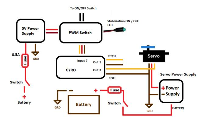
Connect the PWM switch to Input # 7 of the Gyro, and servos to Gyro outputs # 1 to # 4, with the ground wire to the outside of the connectors as shown below:
