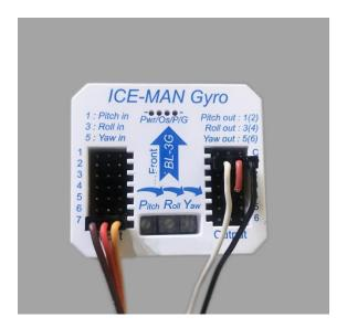
Always connect the ground wire on the outside of the connector (input and output)
