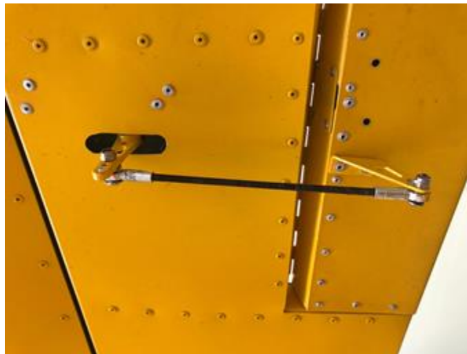
H5 trim tab servo mounted within the elevator control surface
